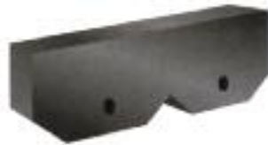
80 DUROMETER RUBBER BLADE (one-piece with "V" notches to conform to belt)
